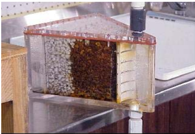
Photograph 2. Horizontal flow (wedge) column.
